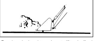
The lift and rollback of the bucket will increase efficiency because...
